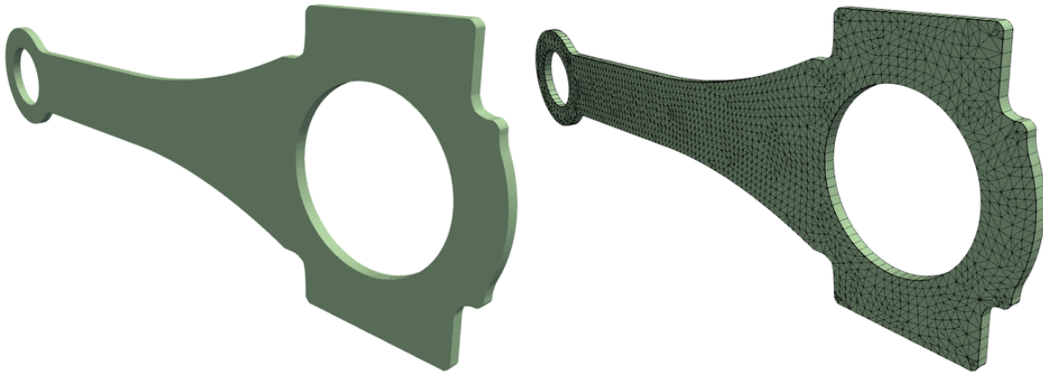
Figure 3.51: CAD and high-order curved prismatic mesh of a mechanical component. The triangular surface mesh is generated without performing mesh enhancement (i.e. diagonal swapping)
