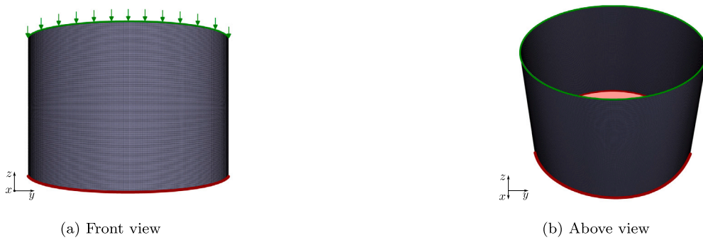
Fig. 15. Presents the thin walled cylinder discretised into {2, 240, 150} thickness, circumferential and length elements respectively for one quarter of the geometry. The cylinder is fixed at the base indicated by the red line and an initial compressive velocity profile v|_{t=0} is applied on the top surface as indicated by the green line and arrows where v|_{t=0} = [0, 0, -80] ms -1 .
